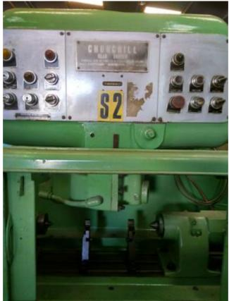
Machine Id 1082 Serial No not available Category **Gear Related Machines** Model gs-12 Country Make churchill England Type of Machine :gear shaver with crowning Year 1980
