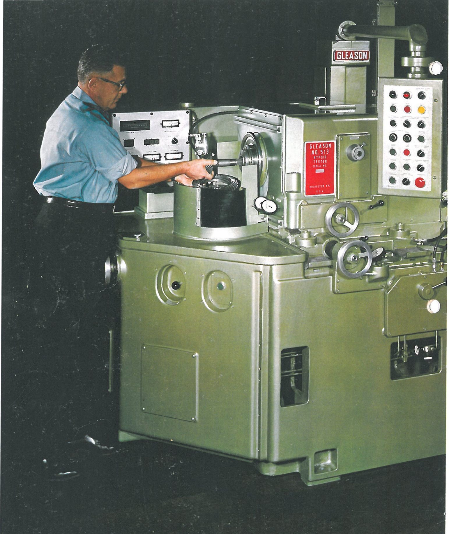
The No. 513 Hypoid Tester represents a technological breakthrough in testing spiral bevel and hypoid gears. It features a unique quality measurement system that automatically identifies gear sets as acceptable or reject, on the basis of running quality. This system eliminates the dependence on human judgment previously required.
